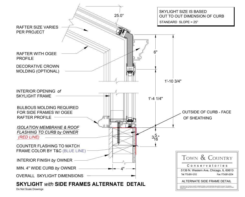
SKYLIGHT SIZE IS BASED **OUT TO OUT DIMENSION OF CURB** STANDARD SLOPE = 25°
