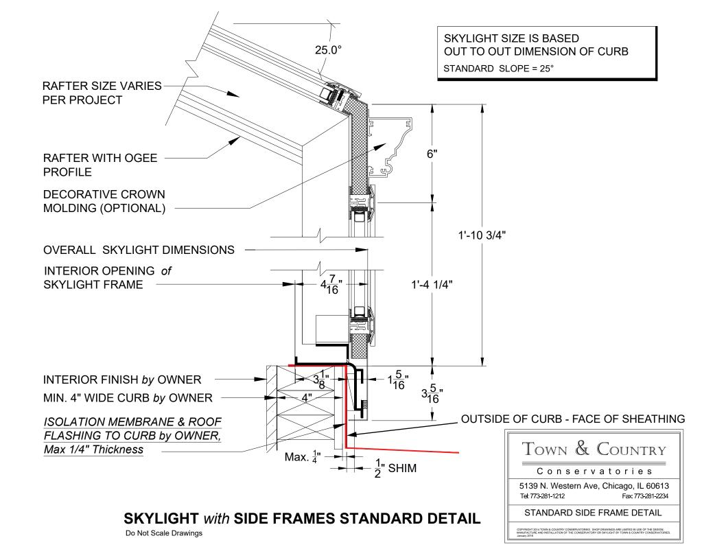
SKYLIGHT SIZE IS BASED OUT TO OUT DIMENSION OF CURB
